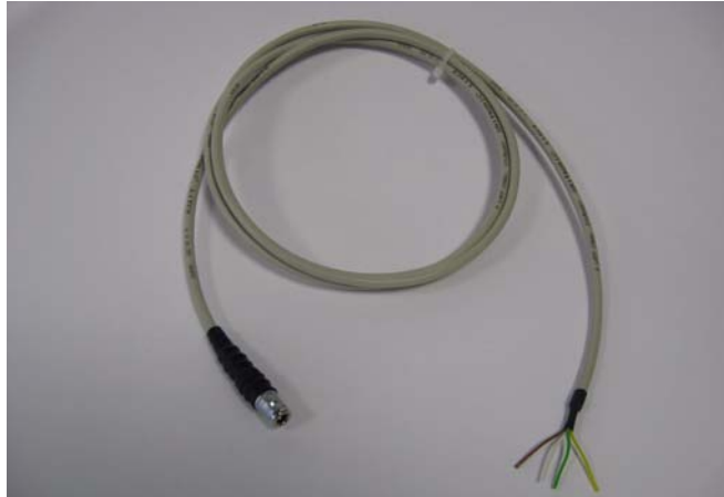
Fig. 6: Connector for interfacing analogue signals to the module
