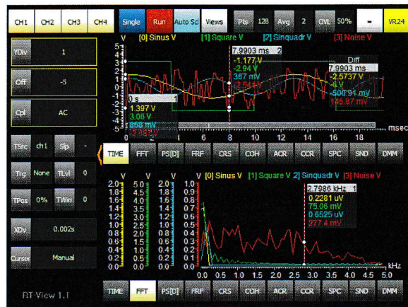
Simultaneous Time and FFT view with multiple Cursors and four channels
