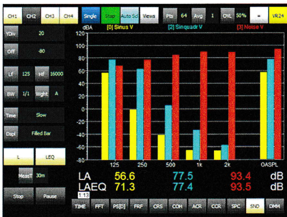
Octave analysis with A-weighting, sound pressure level and equivalent continuous sound pressure level calculation
