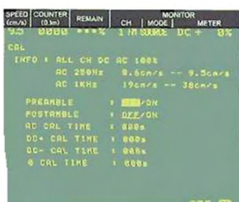
CAL Main Menu Permits programming CAL (calibration voltage) types for automatic recording.
