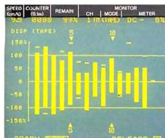
DISPLAY BAR Displays data from all channels at once in bar-graph form.
