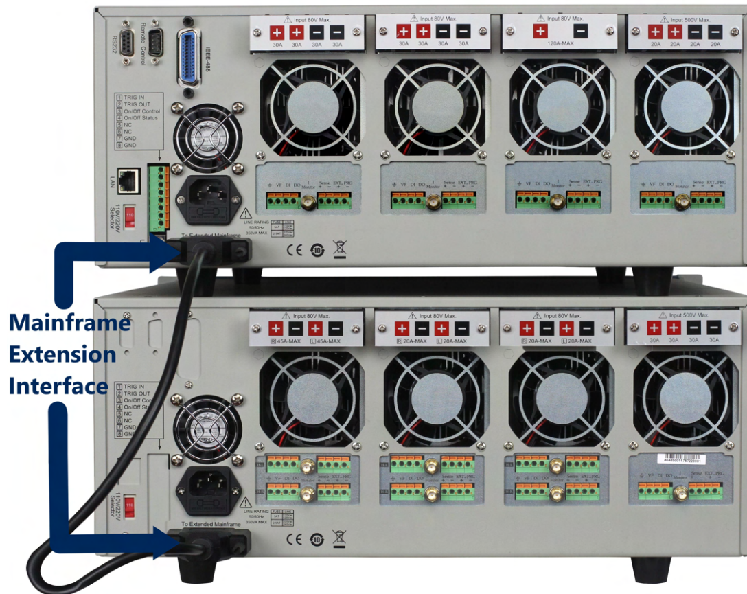
Figure 5.5 Mainframe Extension Connection
