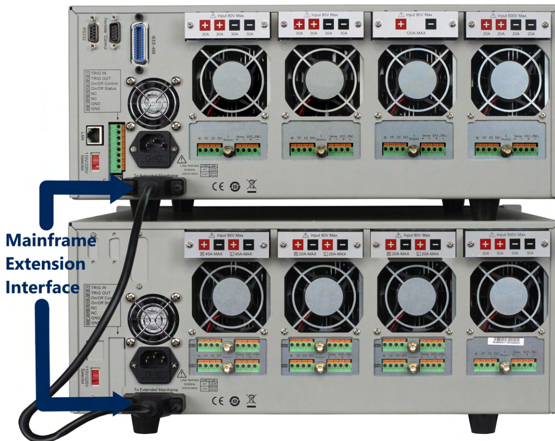
Figure 3.5 Mainframe Extension Connection
