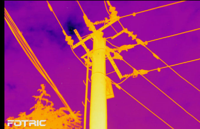
1280*1024 IR resolution (25° lens at 30m distance)
